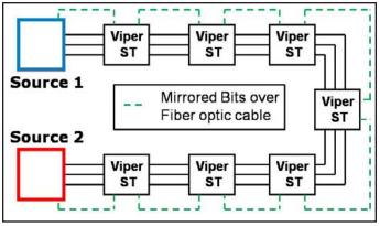
Diagram 1: Single Phase Tripping, Closed Loop
