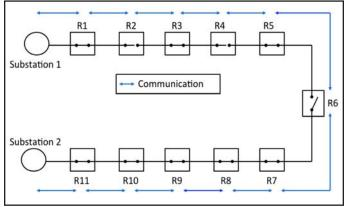
Diagram 2: Three Phase Tripping, Open Loop
