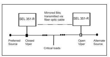
Diagram 3: Voltage Loss Distributed Auto-Transfer Control
